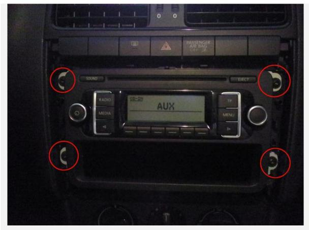
Theses screws can be easily removed with a Torx-Screwdriver (10)
