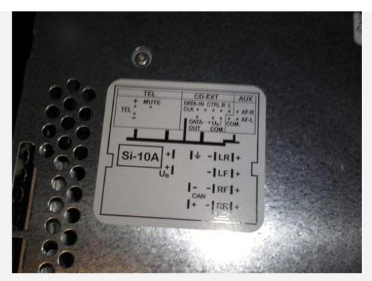
This schema is sticked on the top of the extracted car radio and shows which pins are corresponding to which function or wire. In our case we are interested into the AUX block and the AF-R, AF-L and COM pins.
