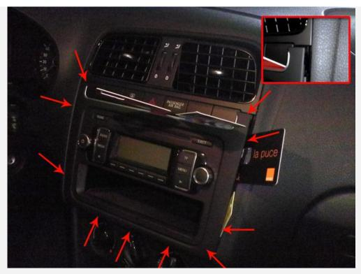
The arrows show where to place your tool in order to reach the clips. Please don't use any screwdrivers because you would scratch the frame and if you make a bad manipulation even the car radio itself.
