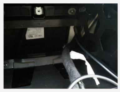
Now you can put the cable along the big Quadlock cable. You can push the cable till it comes out on the bottom of the central console.
