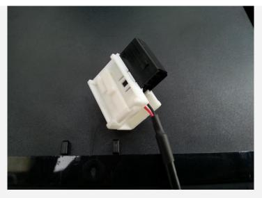
You must remove the white block in order to plug it correctly and without having to disconnect the Quadlock.
