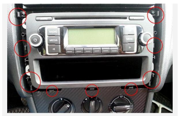
Front view of the car radio with the plastic frame removed. Notice the placement of the clips. The three on the buttons are not very strong, so be careful when you unclips them.
